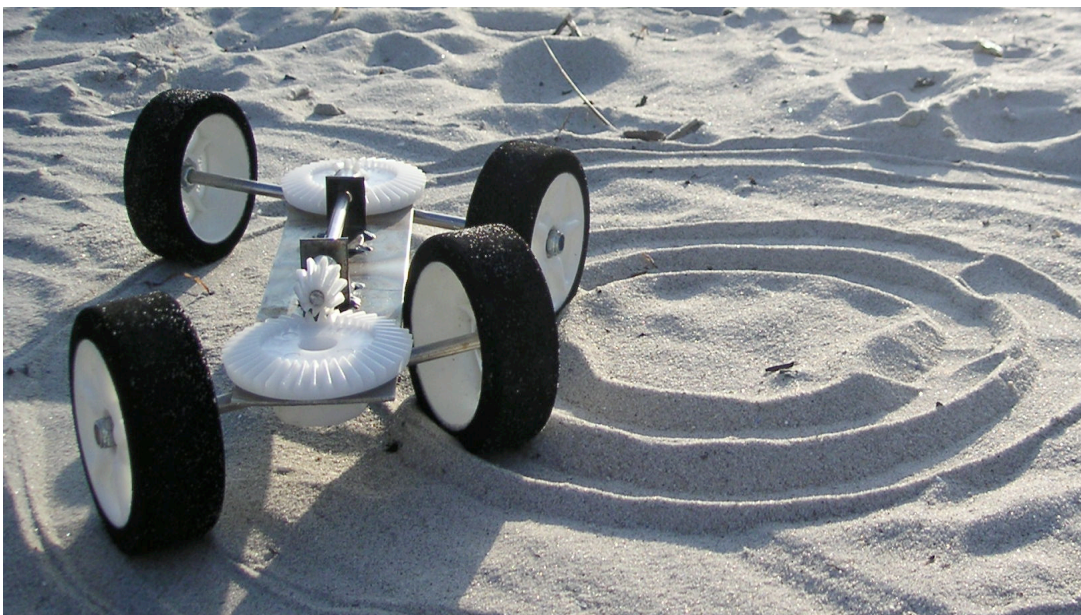
Figure 10: Test of the steering radius of the lawn mover chassis prototype.
